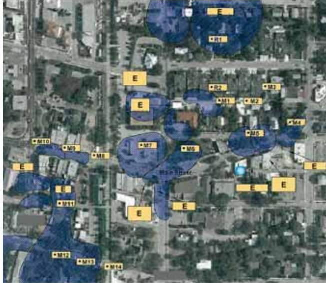
Figure 4: A plan showing the different acoustic zones of the entertainment districts, with ‘M’ and ‘R’ being the receiver locations, and ‘E’ being entertainment venues (source).
